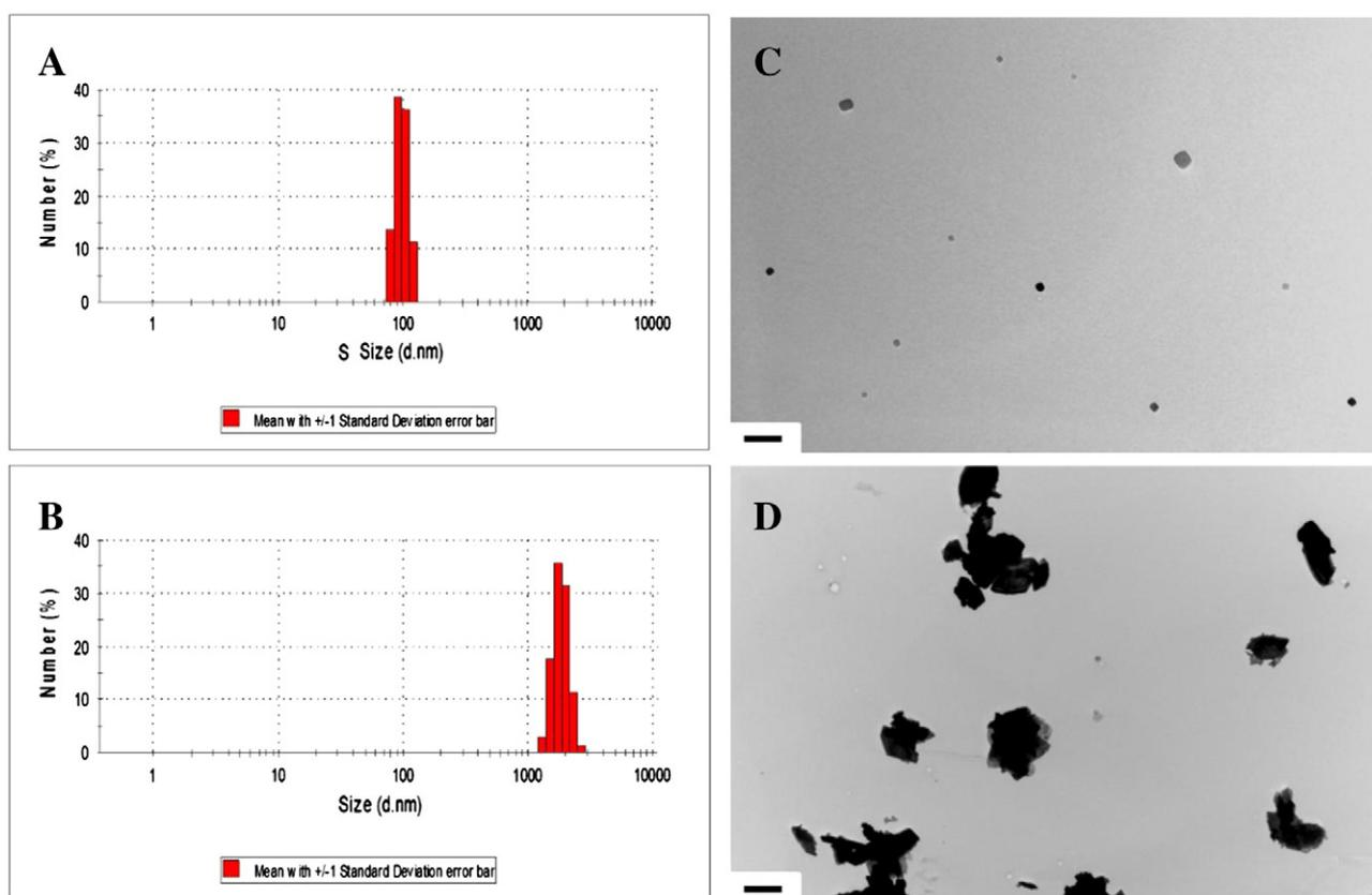
**Fig. 1.** WC-Co particle characterization via dynamic light scattering (DLS) of A) nano-WC-Co and B) micro-WC-Co particles suspended in cell culture media (average size = 98 nm and 3.4  $\mu\text{m}$ , respectively) and representative TEM images of C) nano-WC-Co (scale bar = 500 nm) and D) micro-WC-Co (scale bar = 2  $\mu\text{m}$ ) particles.
