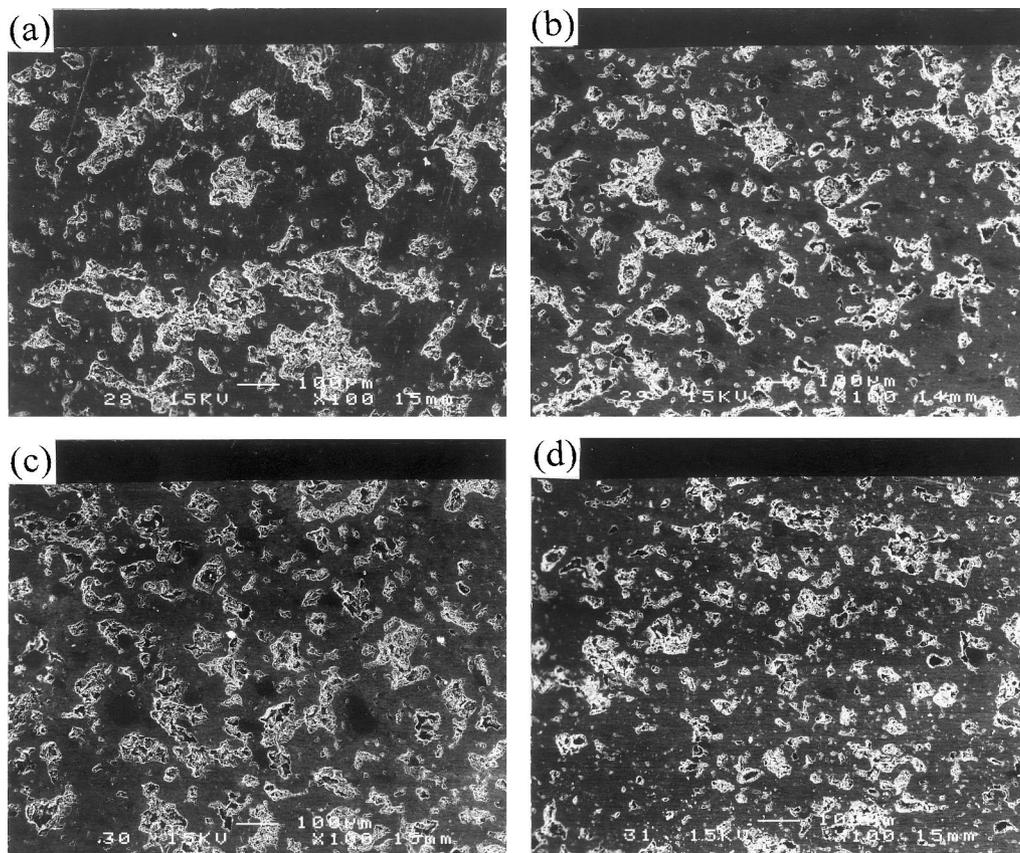
Fig. 1. The micrographs of porous Ni-Ti alloys after sintering at 850°C for 1 h. (a) Sample No. 1; (b) Sample No. 2; (c) Sample No. 3; (d) Sample No. 4.
