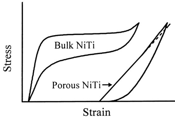
Fig. 4. The typical stress–strain curves of porous and bulk Ni–Ti alloys.
