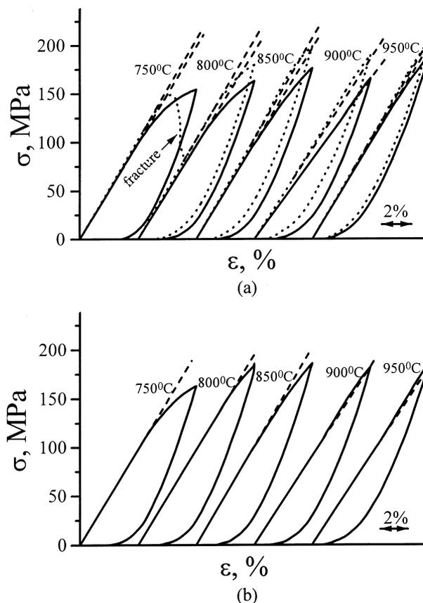
Fig. 3. The stress versus strain diagrams of porous Ni–Ti alloys sintered at various temperatures. The dotted line in (a) is after a second compression of 8%. Dashed direct line indicates the elastic modulus of the linear elastic deformation stage. (a) Sample No. 1; (b) Sample No. 2.
