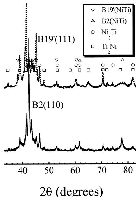
Fig. 2. XRD before and after a compression of 8% of sample No. 4 sintered at 950°C for 1 h. — before compression — — after compression.
