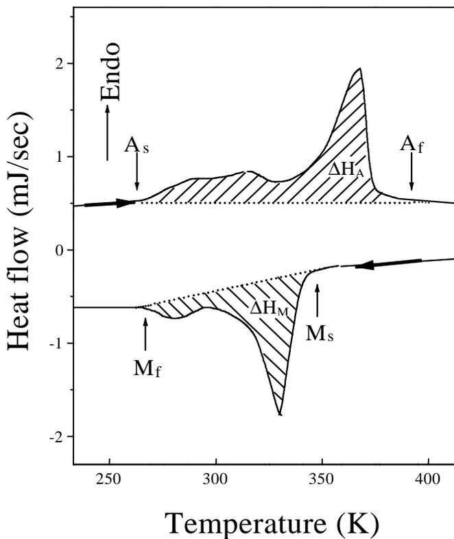
Fig. 1—Schematic DSC curve of porous NiTi alloys.
