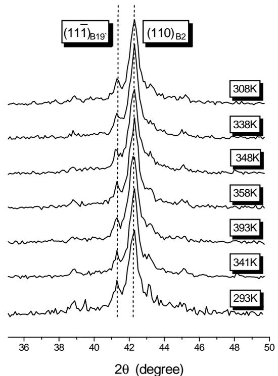
Fig. 2—*In situ* XRD spectra of sample 4<sup>#</sup> sintered at 1223 K for 9h during heating and cooling.
