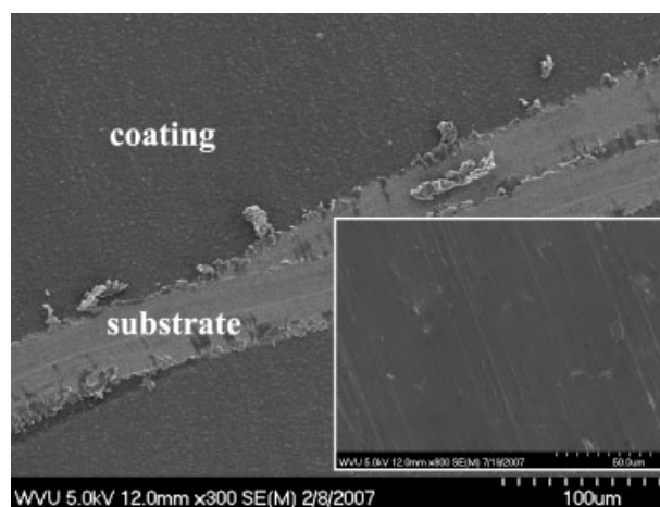
Figure 2. SEM images of stainless steel disc surfaces with and without (the inset) a polypeptide nanocoating. A scratch was made through the coating.
