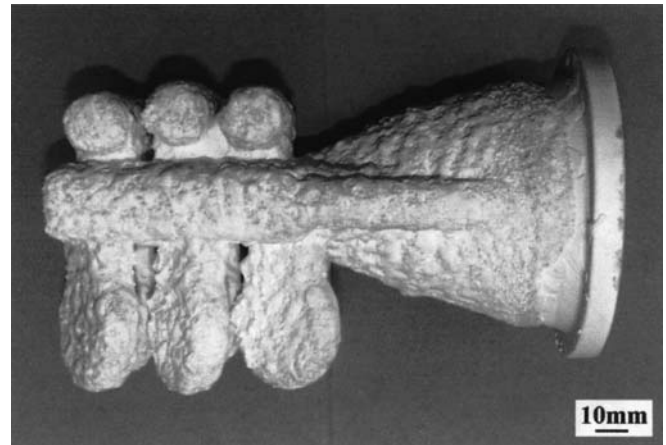
Fig. 3 The ceramic casting mold used in the present study
