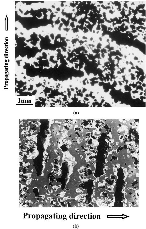
Fig. 5. Optical and SEM micrographs of the longitudinal section of the porous Ni–Ti SMA with a banded structure showing channels along the propagating direction of combustion wave.
