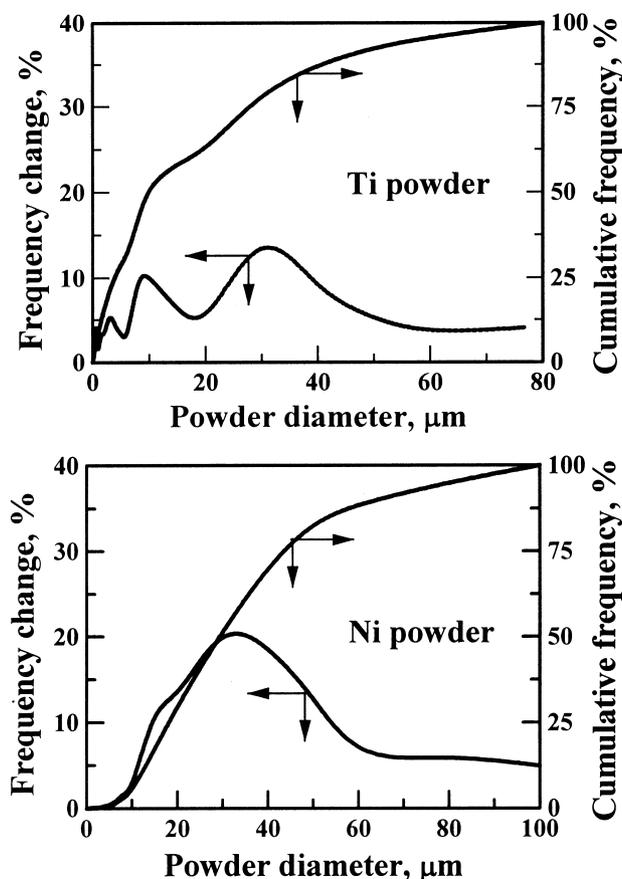
Fig. 1. The characteristics of the elemental Ti and Ni powders.
