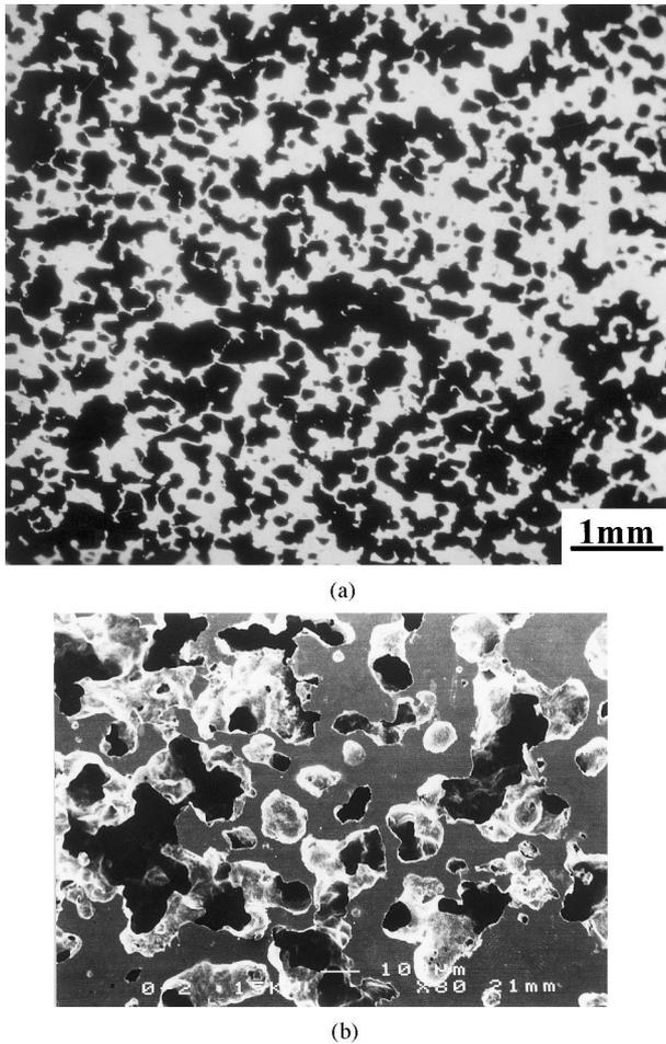
Fig. 4. Typical optical and SEM micrographs of the porous Ni–Ti SMA.
