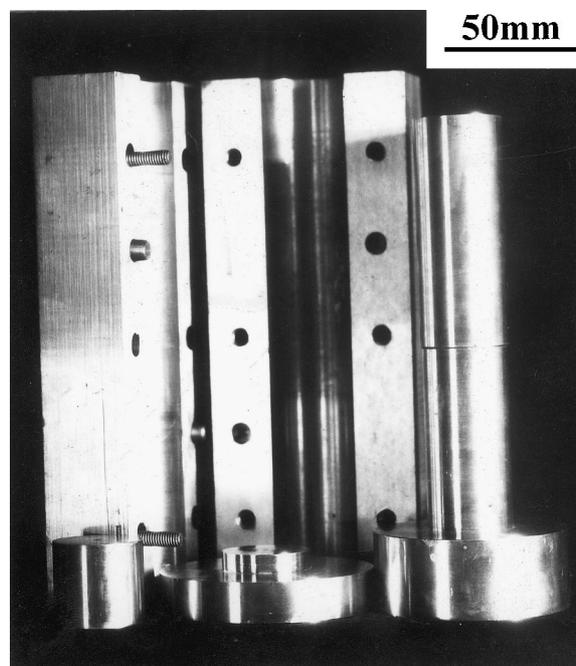
Fig. 2. The cold press die used in the present study.
