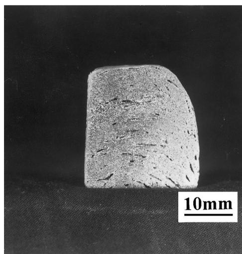
Fig. 3. The macrograph of the longitudinal section of the synthesized porous Ni–Ti SMA.
