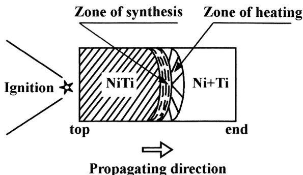
Fig. 7. Schematic representation of the SHS process.
