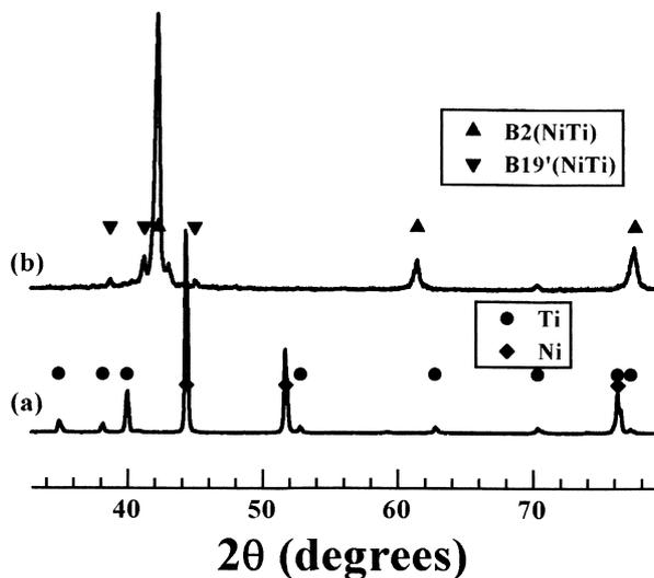
Fig. 6. XRD profiles of the mixed powder and the combustion synthesized porous Ni-Ti SMA.
