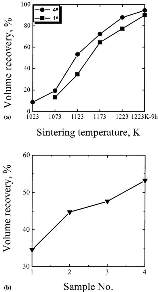
Fig. 5. (a) The volume recovery of porous Ni-Ti materials after sintered at different temperatures. (b) The volume recovery of porous Ni-Ti alloys sintered at 1123 K for 1 h with different TiH<sub>2</sub> addition.
