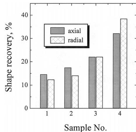
Fig. 4. The shape recovery in axial and radial after prestrain 8% in axial of porous Ni–Ti alloys sintered at 1023 K for 1 h with different  $\text{TiH}_2$  addition.
