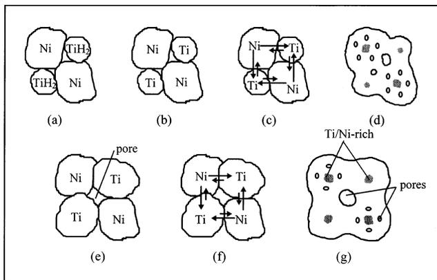
Fig. 6. The schematic diagram of the sintering mechanism model for powder sintering porous Ni-Ti alloys with (a-d) or without (e-g) TiH<sub>2</sub> addition.
