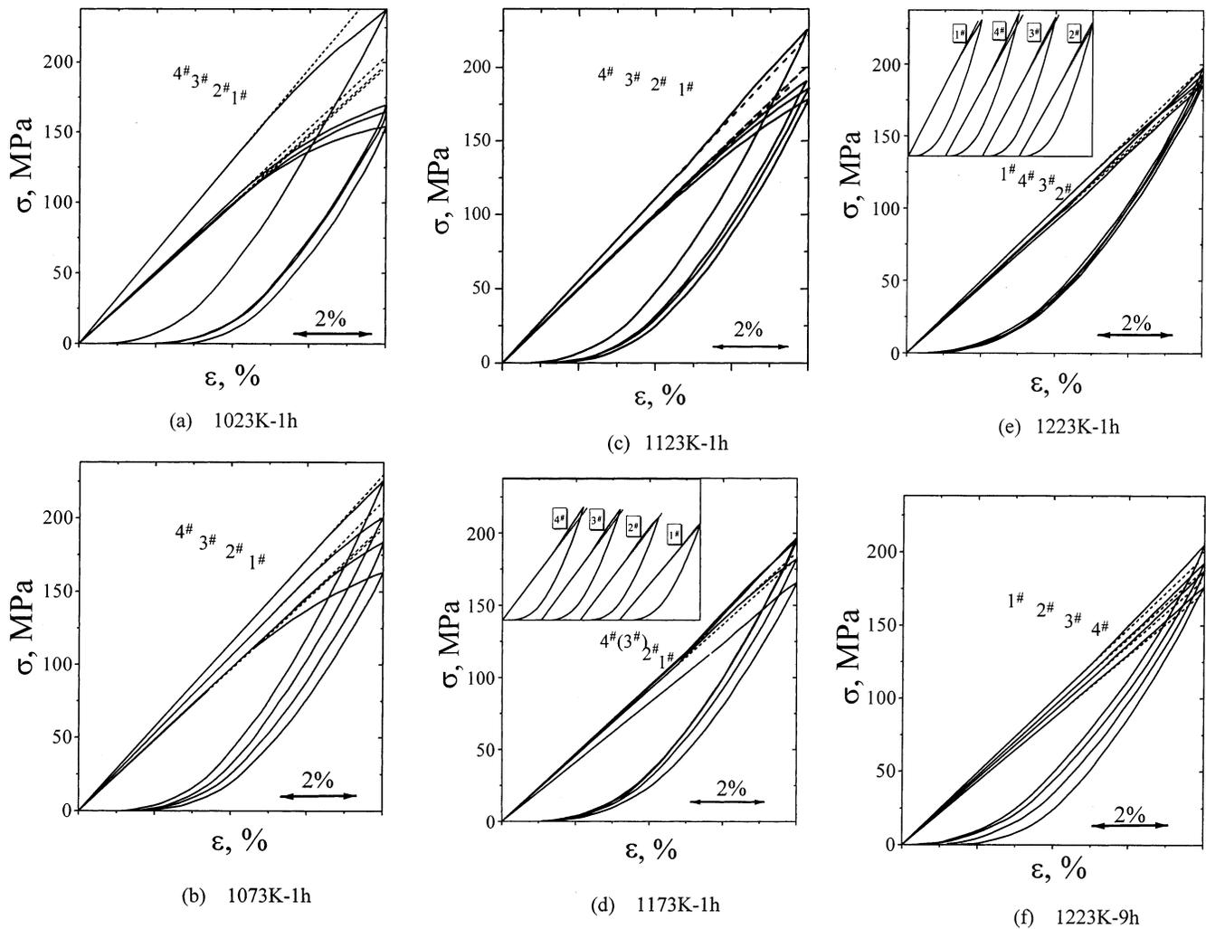
Fig. 3. The stress versus strain diagrams of porous Ni–Ti alloys with different  $\text{TiH}_2$  addition under different sintering conditions ( $\epsilon_0 = 8\%$ ). Dotted lines qualitatively show the Young's moduli. (a) 1023 K, 1 h; (b) 1073 K, 1 h; (c) 1123 K, 1 h; (d) 1173 K, 1 h; (e) 1223 K, 1 h; (f) 1223 K, 9 h.
