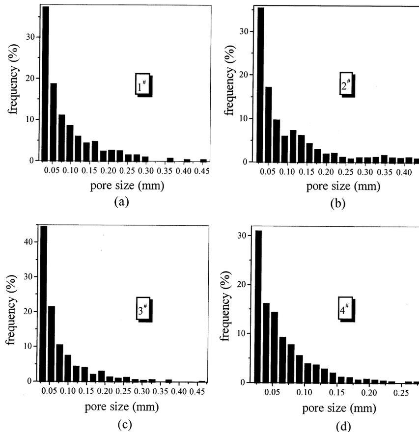
Fig. 2. Pore size distributions of porous Ni–Ti alloys sintered at 1223 K for 9 h with different  $\text{TiH}_2$  addition.
