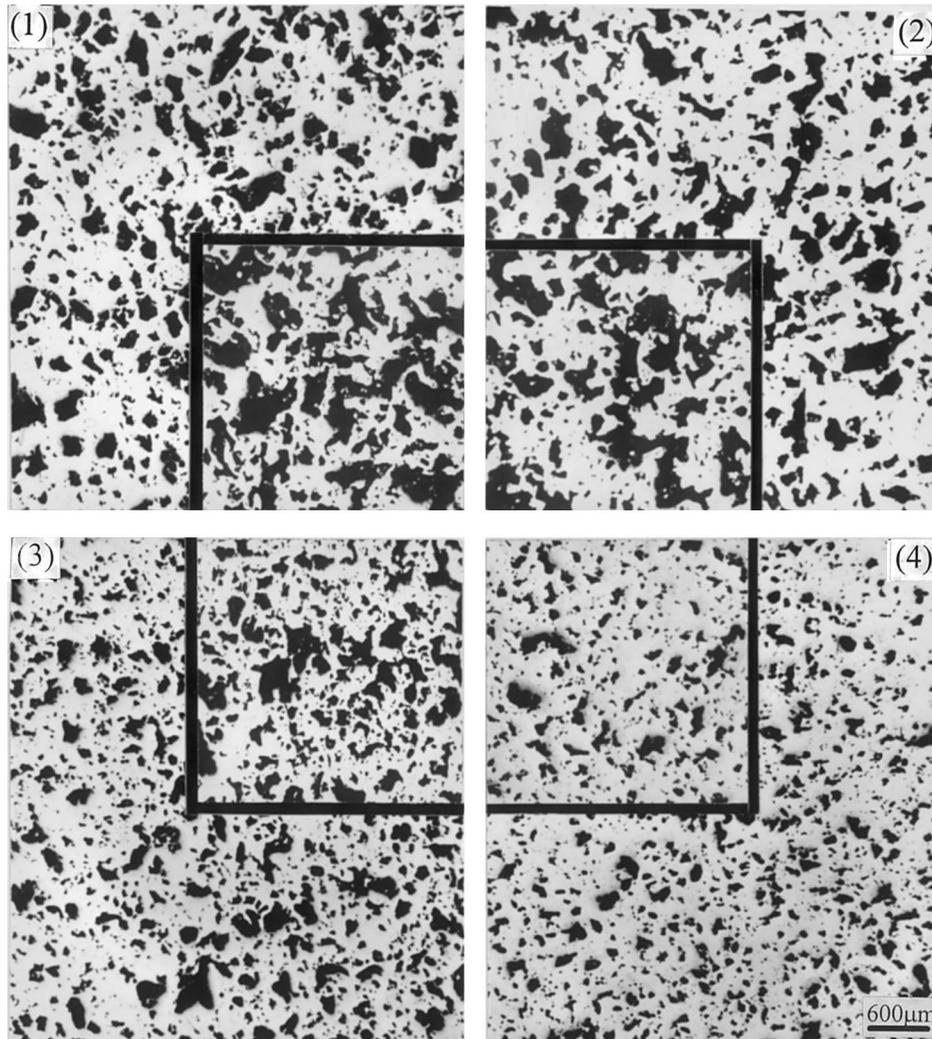
Fig. 1. The optical micrographs sintered at 1223 K for 9 h with different  $\text{TiH}_2$  addition. The insets are the center areas of sintered samples whose pore sizes are different the most from other areas. (1) 1; (2) 2; (3) 3; (4) 4.
