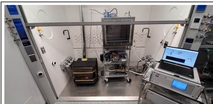
FIGURE D: Military burn pit surrogate generator and aerosol exposure system in the WVU iTOX Inhalation Facility.
